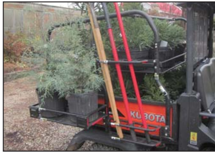
■ RAC "Rapid Access Cargo" System* (RTV-X900 & RTV-X1100C only) V4418 – Long Handle Tool Carrier
